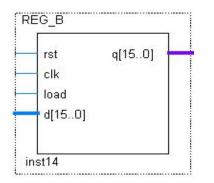
Figure: The register containing load enabling
