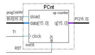
Figure: The alternative circuit of PC
