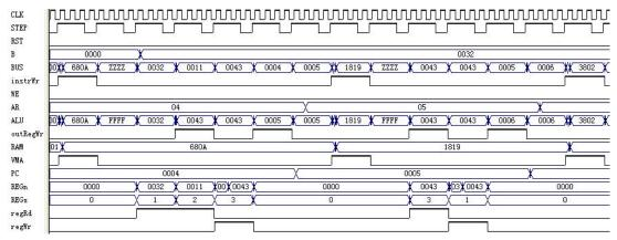
Figure: KX9016 simulation waveform, which includes the timing of ADD command and MOV command
