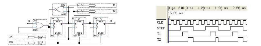
Figure: The circuit and its simulation waveform of beat pulse generator STEP2
