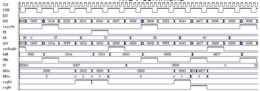
Figure: KX9016 simulation waveform, which includes the timing of STA command and LD command
