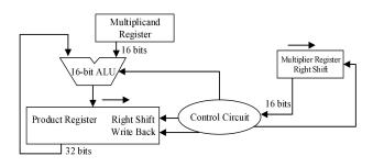
Figure: The hardware implementation of multiplication algorithm 1
