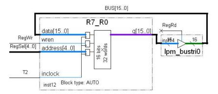
Figure: A circuit that uses LPM\_RAM to replace a register array
