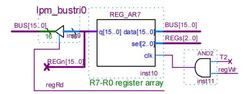
Figure: The register array element and the circuit of three-state control gate
