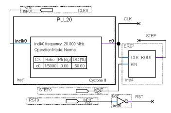
Figure: The circuit scheme for adding phase-locked loop
