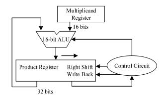
Figure: The hardware implementation of the improved multiplication algorithm 2
