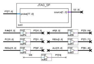
Figure: The connection of the S/P module to the KX9016 port
