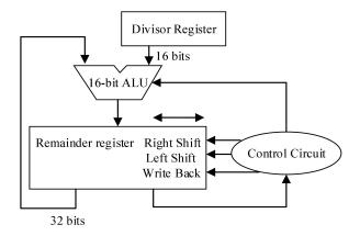
Figure: The hardware structure of division algorithm 2
