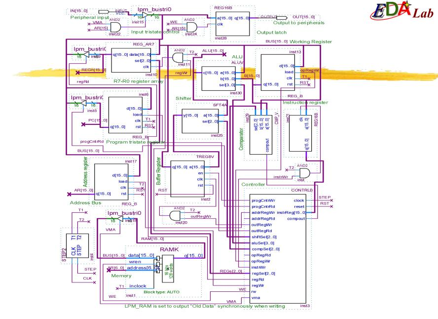
Figure: The structural diagram of the top-level circuit of KX9016v1
