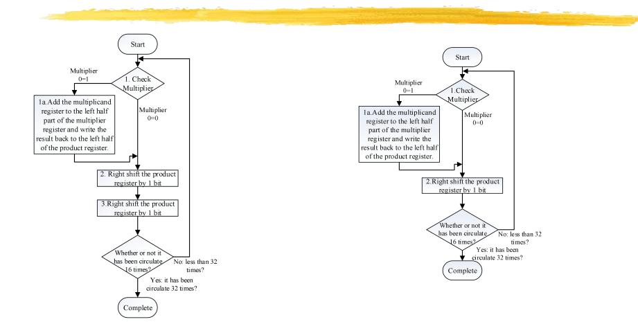
Figure: The flow chart of the multiplication algorithm 1
