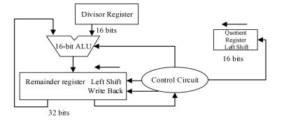
Figure: The hardware structure of division algorithm 1
