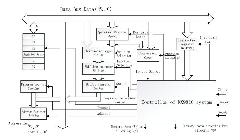
Figure: The top-level structural diagram of 16-bit KX9016v1 CPU
